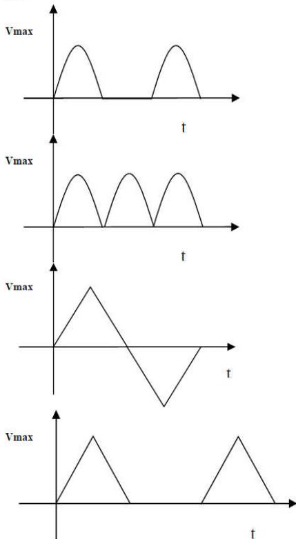
$$V_{moy} = \frac{V_{max}}{\pi}$$
